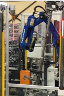
Unmanned inspection equipment judging the acceptability of welds in an instrument panel reinforcement
