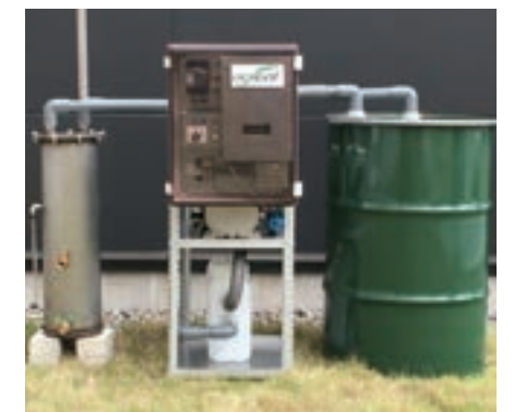
▲aleaf purification, accumulation, and application device for greenhouse cultivation
