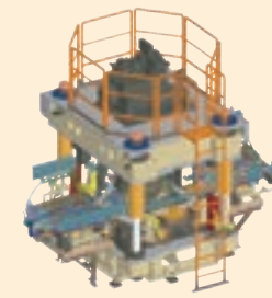
Three dimensional CAD of a hemming device and hemming die
