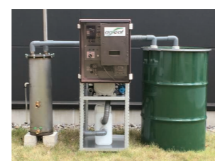
agleaf® CO 2 accumulation and application device for greenhouse cultivation
