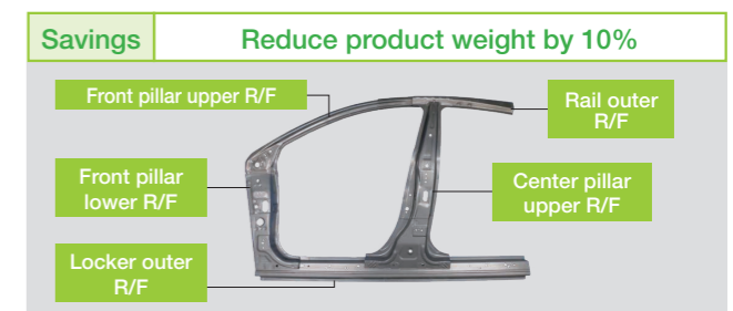
Body parts made with 1470MPa material
