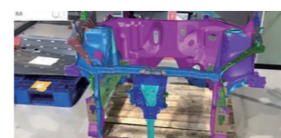
Comparison through overlaying 3D data on actual stuff
