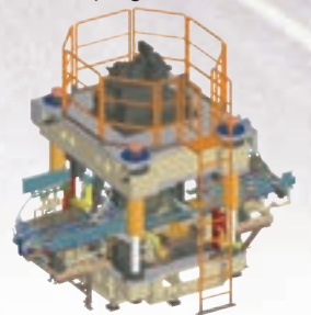
Three dimensional CAD of a hemming device and hemming die
